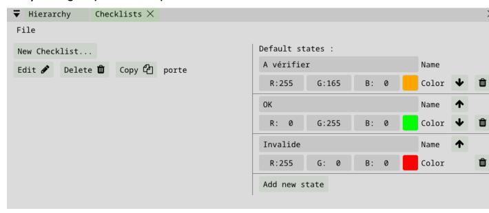
The first status (here "a verifier" = "to be checked") will be the initial status of the objects imported into the checklist when the checklist function is launched in NEXT-BIM Explorer.
