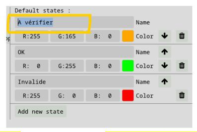
The status evolution in NEXT-BIM Explorer (when you click on an object to be checked in the HoloLens, the object goes from status n°1 "à verifier"="to be checked" to status n°2 "Ok" at the second click the status evolves from "ok" to "Invalid" etc...) corresponds to the order from top to bottom of the statuses in your checklist configuration
