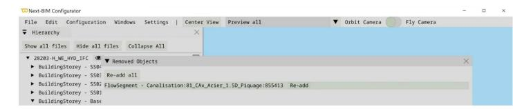
To put the object that was deleted back into the final file, click > "Re-add" on the desired object or > "Re-add all" to put several objects back with one click.
