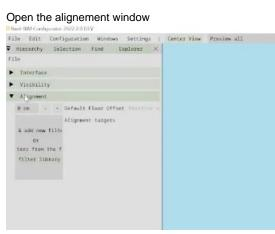
Create & Add New Filter, Add a rule to sort your targets, for example with a name rule if you put "Targets" in the name or a file rule if you created a new .ifc file for these targets.
