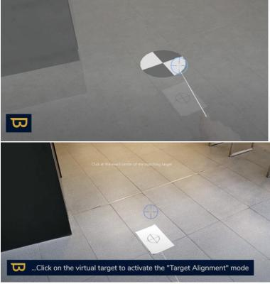
• Aim at the center of the nearby real target and click again (or use voice to say 'select') - the virtual model should now be aligned to the real one.
