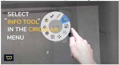
• Then select the desired element - point and click using thumb and pointer finger. The info tool will appear in front of you.
