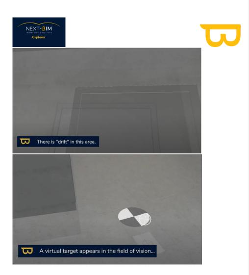
• Click on the virtual target to activate the 'Target Alignment' mode (using your thumb and pointer finger).
