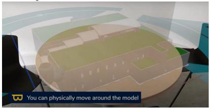
• The horizontal cursors (on a blue or red line) cut the model. Use the same pinching method to cut your model as needed
