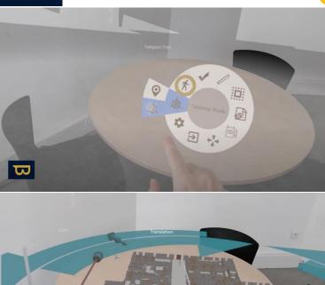
The model keeps the orientation of tabletop mode, so whenever you rotate the model, your immersive mode will also be rotated.
