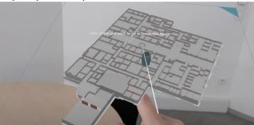
The Teleportation Tool is usable only when model alignment has not been done (in a meeting room for example). Once model alignment has been performed, you can only move around physically.
